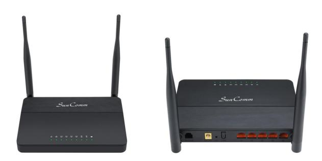
SC-2071MX-4GR 4G LTE WIFI Router includes extended functions which support one 4G card, and 2 FXS ports. This design is not only provide users with a conventional VoIP and routing capabilities, but also allow users to enjoy 4G wireless network anytime. Users can also take SC-2071MX-4GR as a FTP server, to share LAN files, pictures and other resources. Meanwhile, 2 FXS ports can be well adapted to small and micro enterprises, 1FXS for telephone, 1FXS for Fax, no need to add additional equipment.
